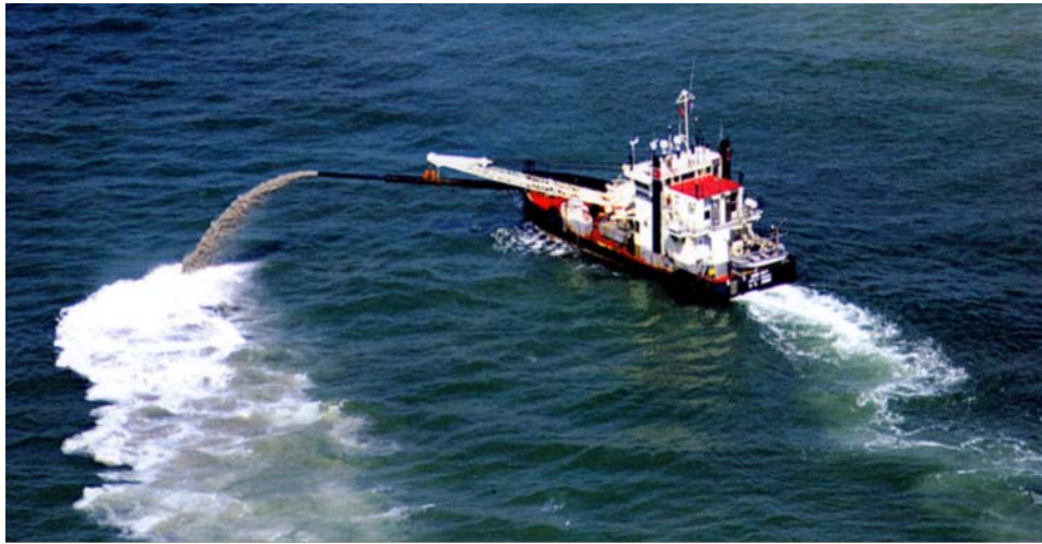
Figure III-14. Typical Sidescaster Dredge
